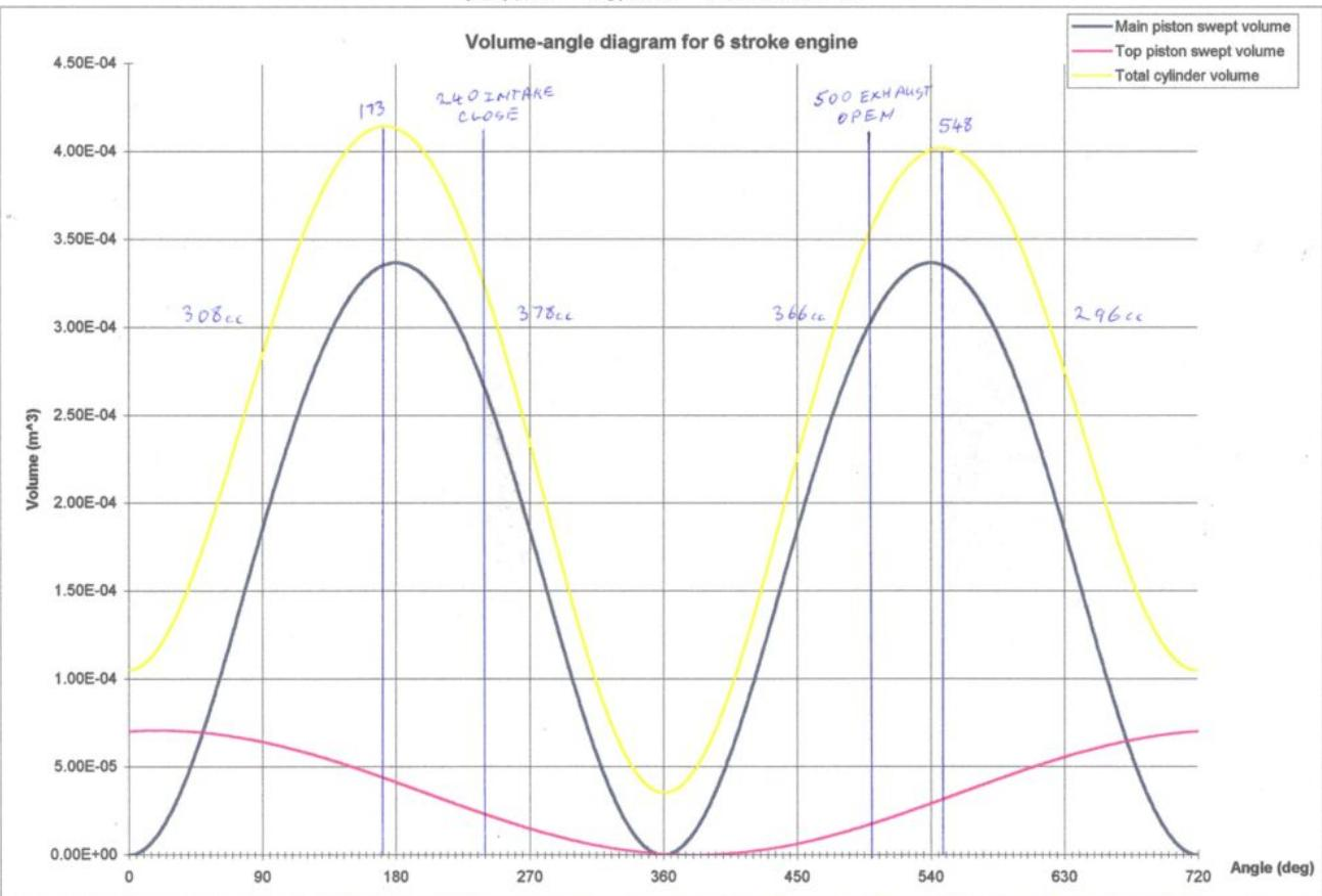
EXPANSION STROKE CHANGE IN VOLUME FROM 360 TO 500 IS GREATER THAN THE CHANGE IN VOLUME OF THE INTAKE STROKE 0 TO 173 AND THE CHANGE IN VOLUME OF THE COMPRESSION STROKE 240 TO 360 AND EXHAUST 548 TO 720
